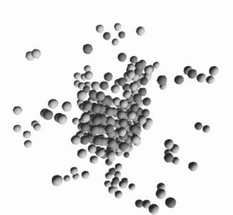
FIGURE 4.2 Snapshot of all solid particles in the r^{-12.5} system at the precritical side of the nucleation barrier, at 25% supercooling ( P = 22.54 , T = 0.75 ). The size of the large solid cluster in the middle is 150 particles.
